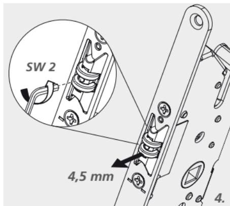
**Please note:** Only to be used with pull handle. Roller latch is retracted via the transmission.
