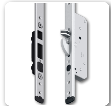
Type 10 automatic secondary locking with latching bolt and steel hook bolt
